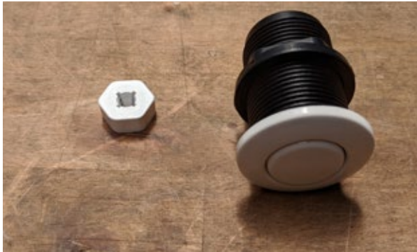
Pneumatic switch of the swim jet
